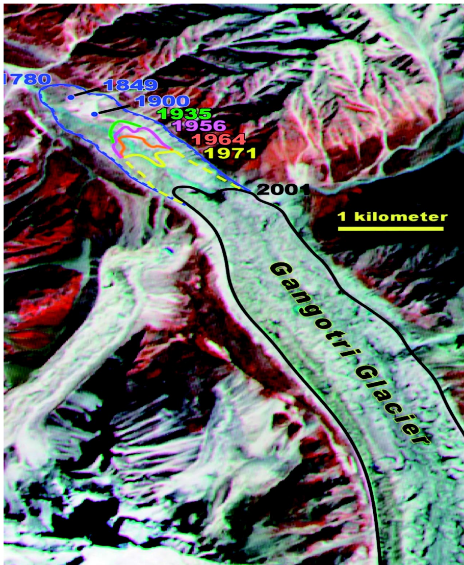
FIGURE 20: Retreat of the Gangotri Glacier (Garhwal Himalayas) snout during the last 220 years
