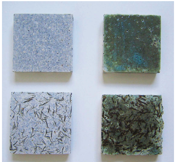
Glazed Concrete Tiles. These tiles used the same glaze but the two lower tiles contain steel fibres. Glaze fired at 1260°C.
