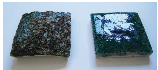
Top: Concrete Tiles with Engobes and for the Tile Below at the Right also with a Transparent Stoneware Glaze. Fired at 1260°C.
