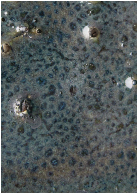
Concrete tile glazed with a stoneware glaze. Fired at 1260 degrees Celsius.
