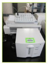
HEWLETT PACKARD 8453 UV-VISIBLE SPECTROSCOPE SYSTEM
