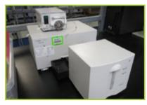
AGILENT 8453 UV-VISIBLE SPECTROSCOPE
