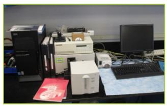
AGILENT 8453 UV-VISIBLE SPECTROSCOPY SYSTEM
