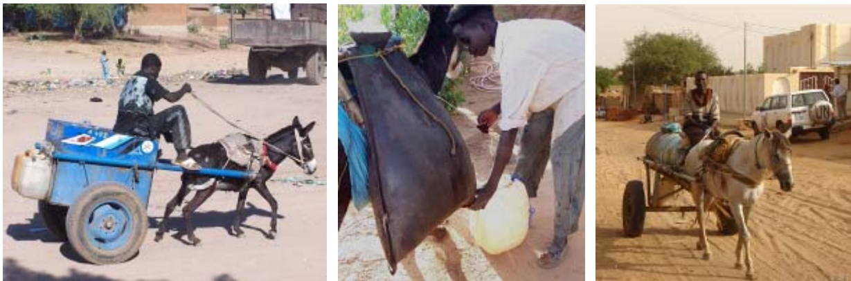
Figure 15: Water distribution in Darfur, Sudan. On the left is the welded donkey-drawn metal tank commonly used for water delivery in Nyala. The middle shows the donkey-borne bladders used for distributing water in El Geneina, and the right shows the horse-drawn tank used in El Fasher. Although all three towns are in Darfur, they each have a different distribution system that is adapted to the local conditions. For example, in El Geneina, the sand is so soft that using a wheeled vehicle to delivery water would be difficult in many areas. You should be aware of differences within and between zones.
