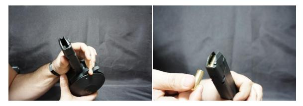
While keeping the spring compressed, slide a cartridge primer, end first into the gap created.
