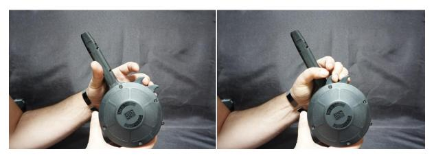
With an empty magazine, turn the loading lever counter clockwise from the front to compress the spring.
