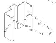
**MULLION:** A metal clip or angle in either 1 or 2 pieces, secured to the floor in which mullion is then positioned over.
