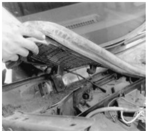
Fig. Fig. 6: Removing the air inlet screen assembly - heater core removal
