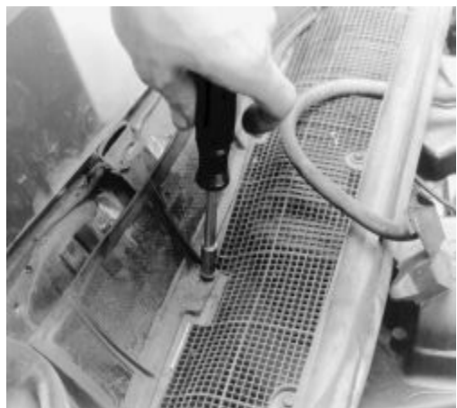
Fig. Fig. 4: Removing the air inlet screen retaining screws - heater core removal
