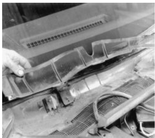
Fig. Fig. 5: Removing the air inlet screen retaining screws - heater core removal
