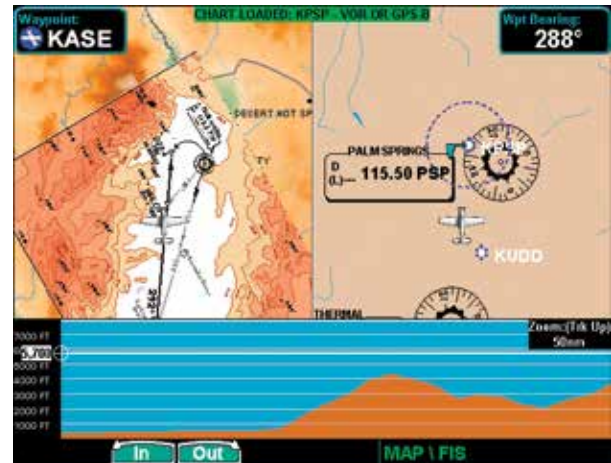
Split Screen showing Custom Map and FIS pages along with the Vertical Profile
