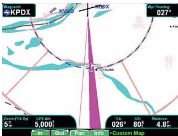
ILS for currently tuned approach by SL30
