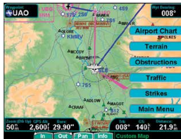
Custom Map page with Airport Charts, Terrain, Obstructions, Traffic, and Storm Cells Menu Items (Page 5)
