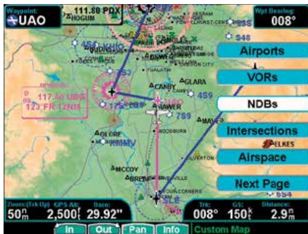
Custom Map page with NDBs, Intersections, and Airspace selected with Menu Items (Page 2)
