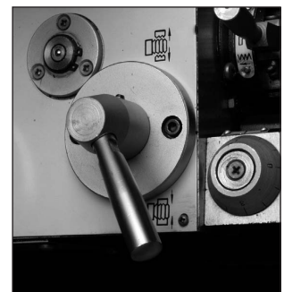
Figure 7.06 Longitudinal Fine Feed Handwheel (Left) Half-Nut Engaged (Right)
