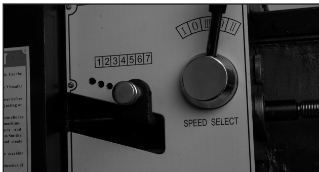
Figure 10.02 Selector Lever (1-7) and Selector Lever (I-III) engaged
