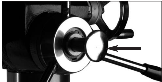
Figure 7.02 Mill/Drill Press Clutch pulled out engaging the Drill Press
