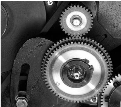
Figure 5.05 Brush a thin layer of lithium grease over the gear quadrant in the pulley box
