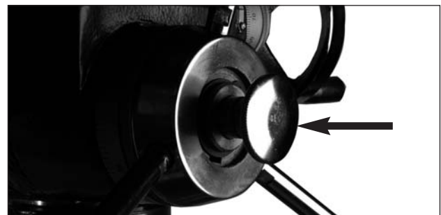
Figure 7.03 Mill/Drill Press Clutch pushed in engaging the Drill Press
