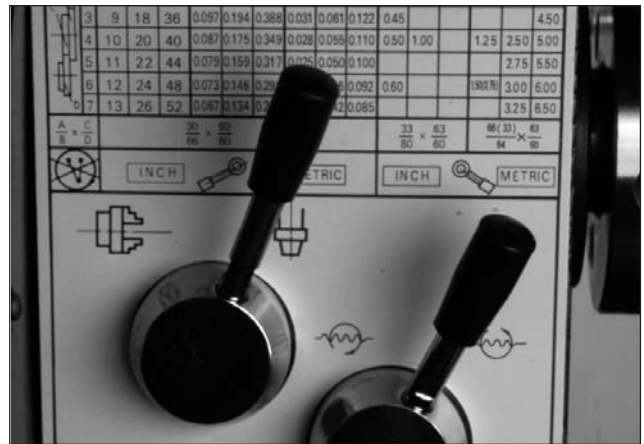
Figure 9.01 Always engage the Powerfeed Function lever to the appropriate operation
