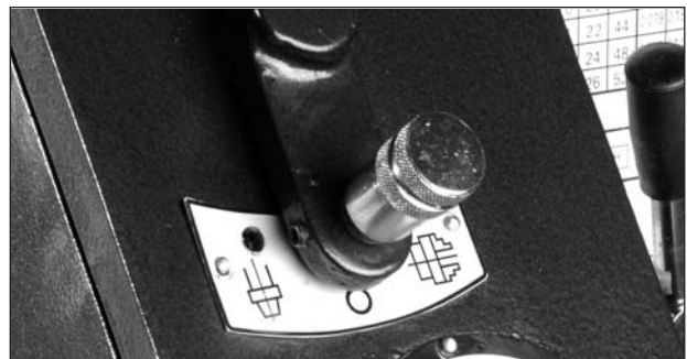
Figure 7.01 Lathe/Mill Clutch Shown in the Neutral Position
