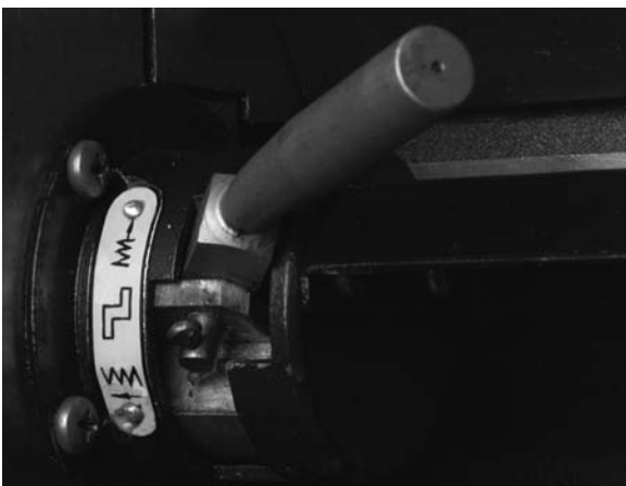
Figure 9.02 Powerfeed Engagement Lever Shown with Y-Axis powerfeed engaged
