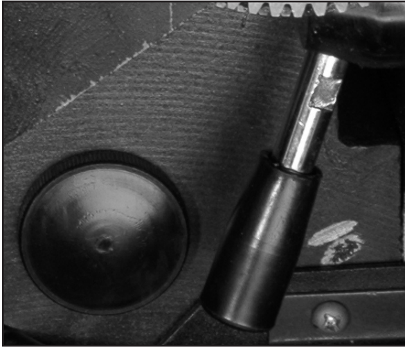
Figure 10.04 Inch/metric Selector located inside the pulley box
