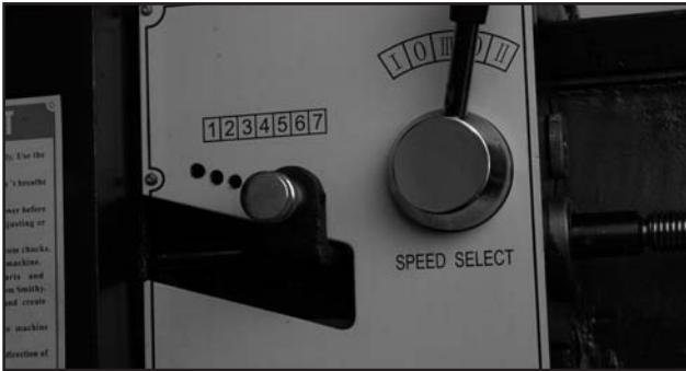
Figure 9.02 Selector Lever (1-7) and Selector Lever (I-III) engaged
