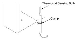
Figure 5 - Attaching Thermostat Sensing Bulb
