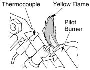
Figure 24 - Incorrect Pilot Flame Pattern
