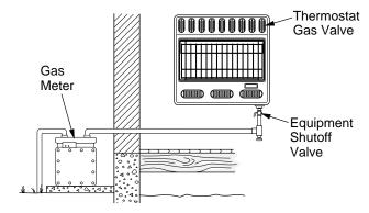
Figure 17 - Checking Gas Joints for Natural Gas
