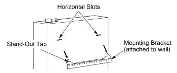
Figure 11 - Mounting Heater Onto Mounting Bracket
