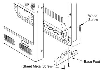
Figure 13 - Installing Base Feet
