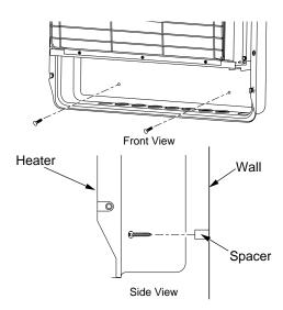
Figure 12 - Installing Bottom Mounting Screws
