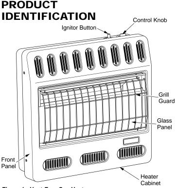
Figure 1 - Vent-Free Gas Heater
