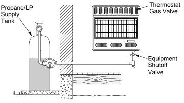
Figure 18 - Checking Gas Joints for Propane/LP Gas
