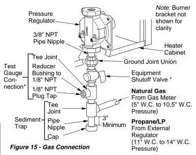
\* A CSA design-certified equipment shutoff valve with 1/8" NPT tap is an acceptable alternative to test gauge connection. Purchase the optional CSA design-certified equipment shutoff valve from your dealer. See *Accessories*, page 27.
