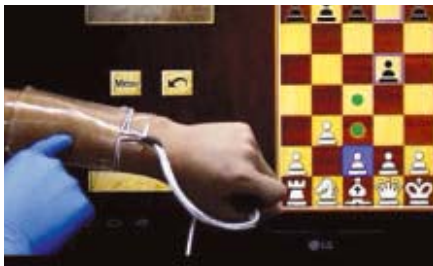
Researchers stretched a flexible touch panel on an arm and used it to play chess.
