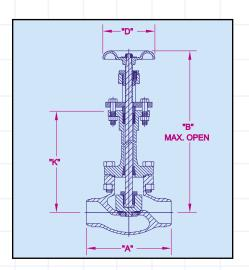
Pressure rating 300 PSIG non-shock cold Temperature rating +150° F to -325° F Dimensional Data All dimensions are in inches
