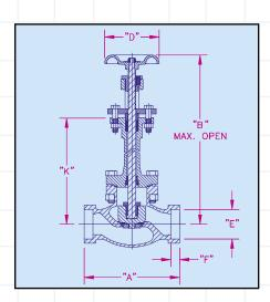
Pressure rating 400 PSIG non-shock cold Temperature rating +150° F to -325° F Dimensional Data All dimensions are in inches
