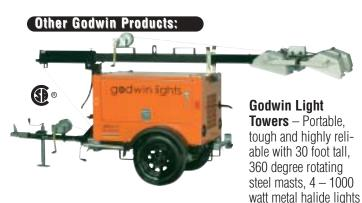
cover 5 - 7 acres. Standard 4 point outrigger stance is capable of withstanding 65 mph winds. Godwin Light Towers are easy to use; engineered for one person set-up and breakdown.
