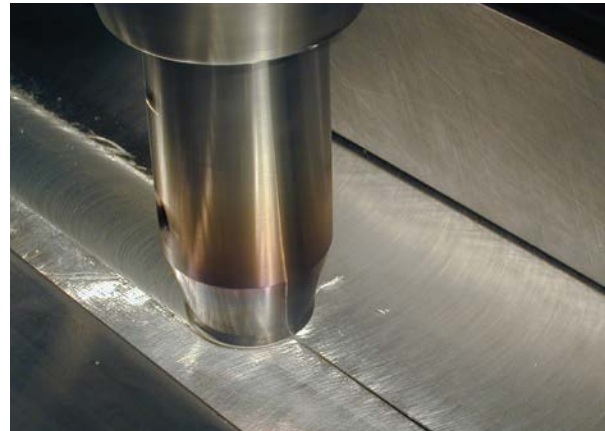
CTC has a long history of creating advancements in engineering and manufacturing, including innovations in friction stir welding, which are being leveraged in a project to manufacture armored vehicle prototype hulls for the U.S. military.
