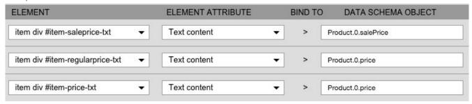
Open **custom.js** and in the initItemDisplay function (which is called for each feed item), pass a reference to each of these three text fields into this function on common.js:
