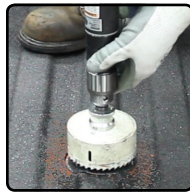
Use the pilot hole for error-free drilling
