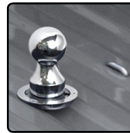
Ball up, ready for coupling
