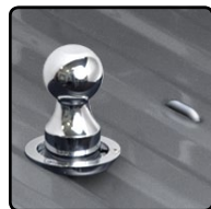
Ball up, ready for coupling
