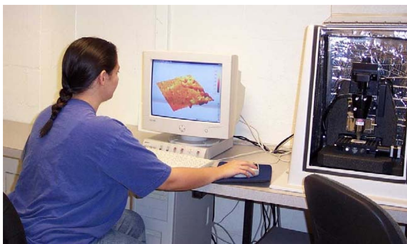
Quesant Atomic Force Microscope is used both as a teaching and as a research tool.
