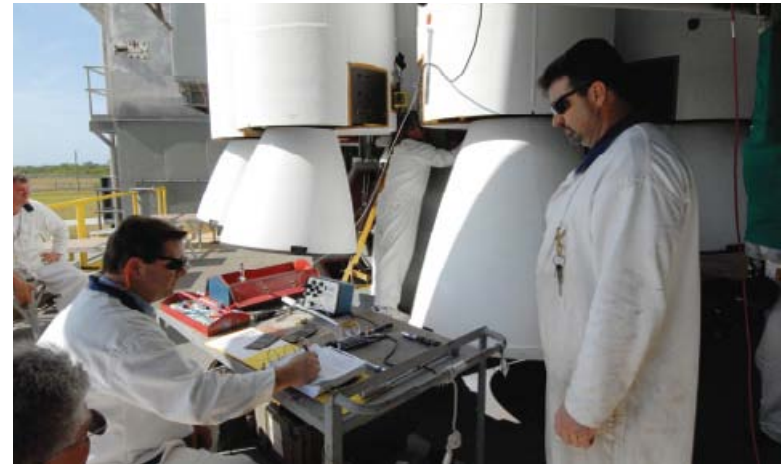
At Cape Canaveral Air Force Station in Florida, technicians check the list of activities completed on the mating of the nine solid boosters to the Delta II rocket for the launch of NASA's Gamma-ray Large Area Space Telescope (GLAST). NASA acquires vehicles like the Delta II from commercial providers to launch robotic space exploration missions. (Photo: T. Cryder/NASA)
