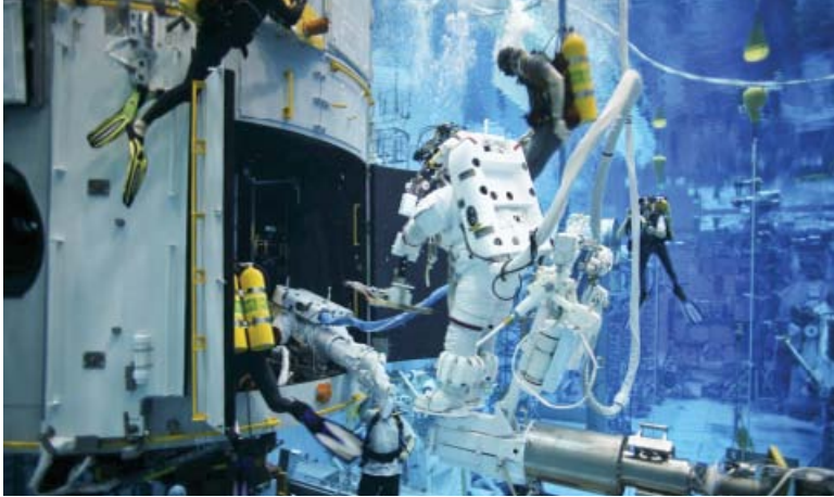
Servicing Mission 4 astronauts practice on a Hubble Space Telescope model underwater at the Neutral Buoyancy Lab (NBL) in Houston under the watchful eyes of NASA engineers and safety divers. To make the most of each spacewalk and ensure astronaut safety, repair tasks are meticulously planned, choreographed, and rehearsed in the NBL so that there will be few or no surprises when the astronauts work on orbit with the real telescope. (Photo: NASA)
