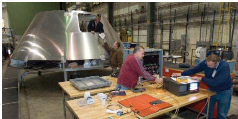
Technicians at the Dryden Flight Research Center prepare for systems installation on an Orion boilerplate crew capsule, which will be used for launch abort testing. NASA has distributed work for Constellation Systems to take advantage of each Center's unique research and engineering capabilities and to use existing workforce and facilities to best advantage. (Photo: T. Landis/NASA)
