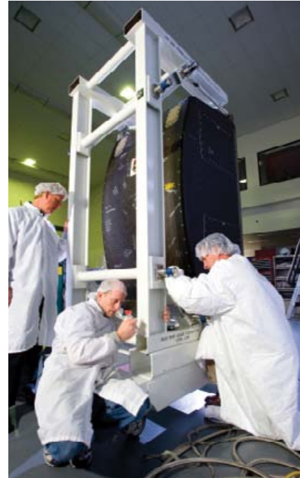
Engineers at Marshall Space Flight Center prepare one of the two ISS Water Recovery System racks for transport to Kennedy Space Center for final flight preparations. The racks, part of the Regenerative Environmental Control and Life Support System, are key to accommodating a crew of six aboard the ISS, and meeting one of NASA's outcomes for the ISS program. (Photo: D. Higginbotham/NASA)
