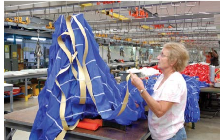
Workers at Kennedy Space Center's Parachute Refurbishment Facility prepare a parachute for an upcoming test. NASA will use the final parachute design to return the Ares I rocket and Orion spacecraft to Earth. Kennedy has transitioned many of the workers from the Shuttle Program as that program winds down and the Constellation Systems Program moves forward. (Photo: K. Shifflett/NASA)
