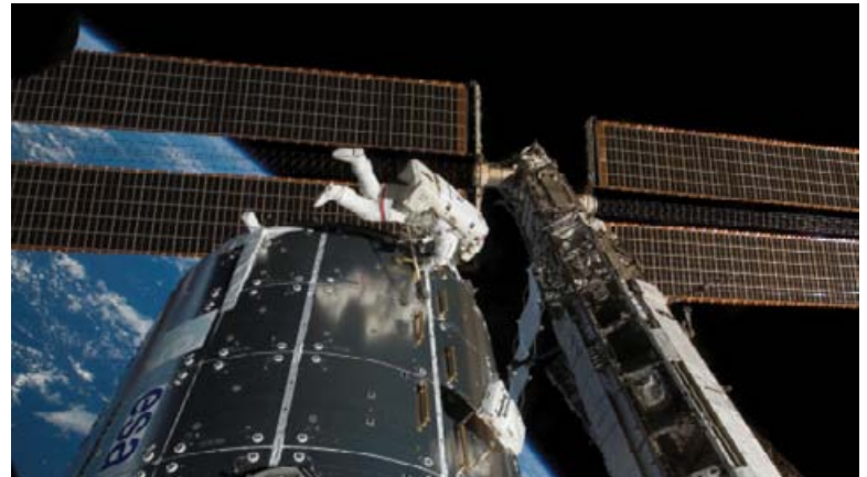
Rex Walheim, mission specialist for STS-122, installs handrails on the outside of the European Space Agency's Columbus laboratory, which was installed on the ISS in February 2008. NASA uses careful program planning and budgeting to keep ISS construction, including launch of International Partner elements, on schedule for completion by the Shuttle fleet's retirement in 2010. (Photo: NASA)
