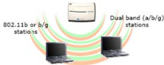
Figure 12 – Simultaneous 802.11a and 802.11g Dual Radio Support (HP Procurve Networking, Planning a Wireless Network)
