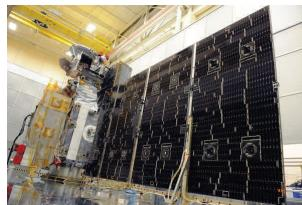
The GPM Core Observatory's two solar panels provide power for all the satellite's systems by converting sunlight into electrical energy.
