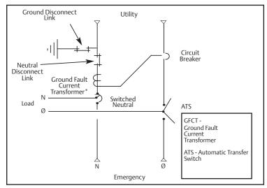
One line diagram of a typical service entrance rated transfer switch available in Solid, Switched or Overlapping Neutral
