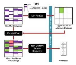
Fig. 6. Schematic of our closest point algorithm showing the inter-communication between the CPU and GPU. The vertical bars represent the range of minimum and maximum distances from the point to the bounding box.
