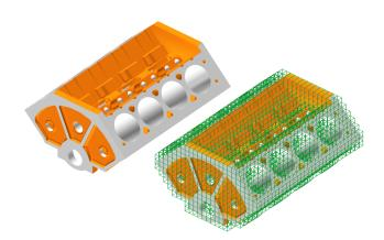
Fig. 14. A complex model and its voxel representation. We store the surfaces that intersect with a particular voxel to accelerate the minimum distance computation.
