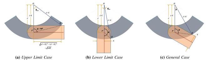
Fig. 18. The three different cases that can arise when the closest point computed is on the edge of the triangle.
