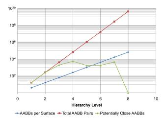
Fig. 12. Plot showing the actual number of AABB pairs compared during a typical minimum distance computation. The number of pairs being tested in parallel remains almost constant after level 3 of the hierarchy. Note logarithmic scale used for the y-axis.
