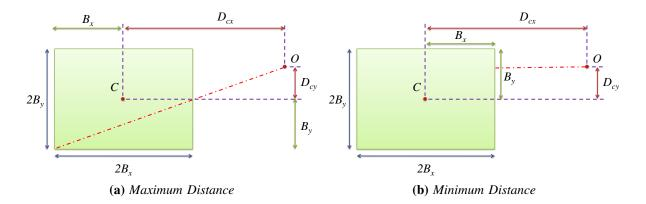
Fig. 7. Efficiently computing the maximum and minimum distance between a point and an AABB. The example shown here is for the 2D case, but the method can be extended to 3D. See Equations (5) - (12).
