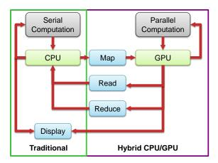
Fig. 3. Schematic showing our hybrid framework that extends traditional geometric computations to use the GPU as a coprocessor to perform some parts of the computations in parallel.
