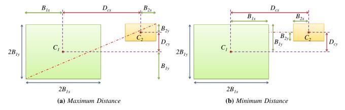
Fig. 11. Computing the maximum and minimum distance between two AABBs. The equations are similar to the point-AABB distance case. See Equations (13) - (20)
