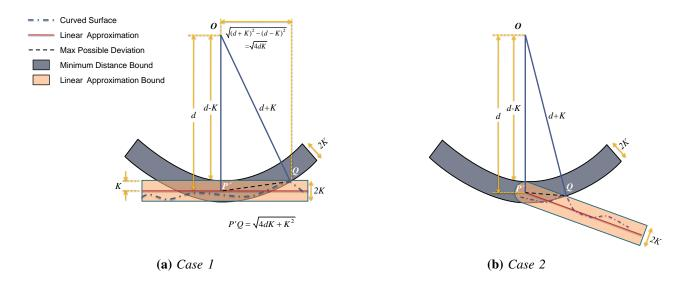
Fig. 9. Illustration to evaluate the bound for the computed closest point location when the closest point on the plane lies either (a) inside or (b) on the edge of the triangle approximating the surface.
