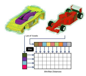
Fig. 15. We map the list of voxels of one object to the rows and the other object to the columns of a 2D texture to compute the minimum and maximum distances between the voxels.
