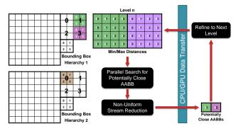
Fig. 10. We perform minimum distance computation between two NURBS surfaces with the help of AABB hierarchies for both the surfaces. We compute a list of potentially close bounding-boxes at each level using the GPU and then refine on the CPU until we reach a set of potentially close boundingboxes at the lowest level.
