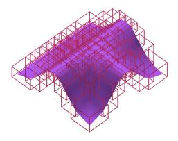
Fig. 4. Surface bounding-boxes constructed from points evaluated on a NURBS surface.
