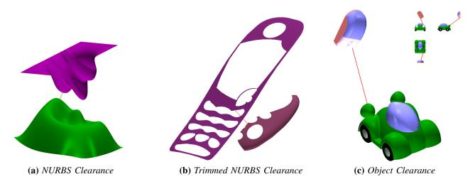
Fig. 1. Minimum distance/closest point computations between NURBS surfaces and complex CAD models accelerated using the GPU.
