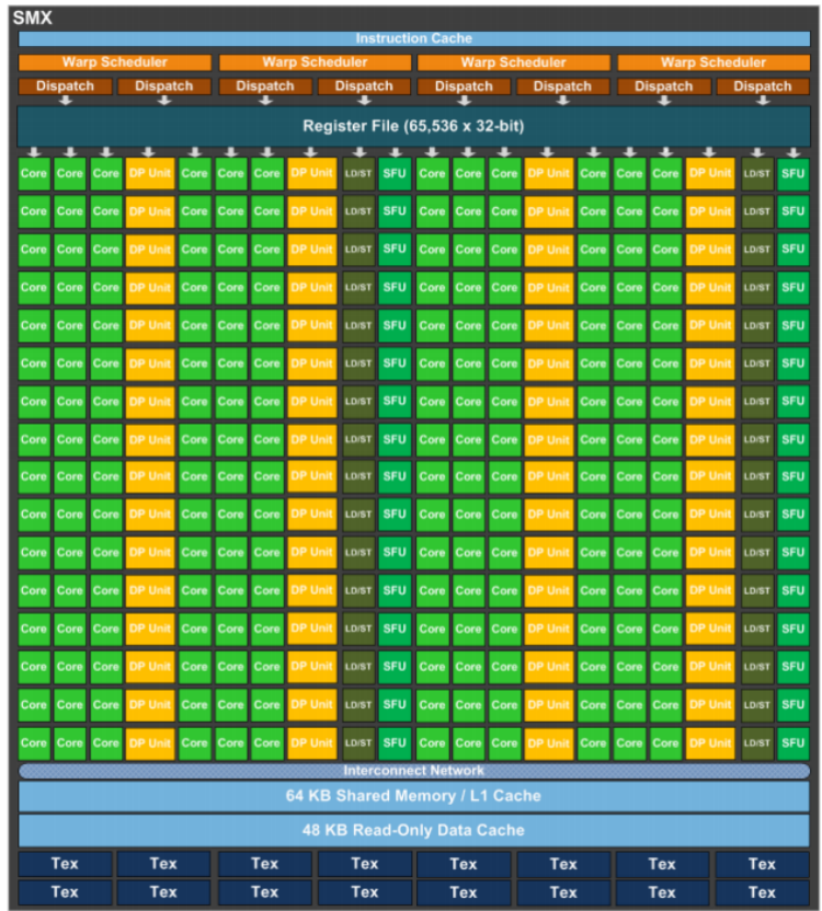
Figure 2: The Kepler Architecture
