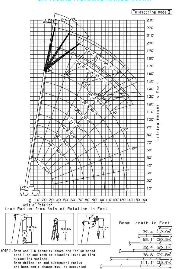
for when applying load to hook.
