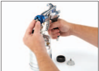
1 Remove front air cap and nozzle
