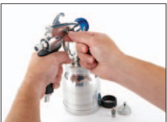
2 Slide trigger lever to release needle
