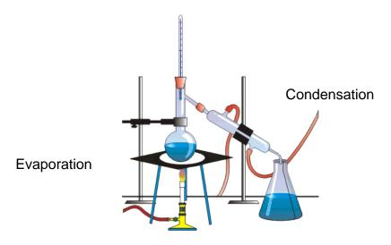
The solution is heated so the solvent evaporates. Once it reaches the top of the flask it begins to cool and condense. The condensing solvent enters the tube and condenses into the flask on the side. Once all the solvent has evaporated/condensed the solute will be left in the original flask and the solvent will be in the flask on the right.
