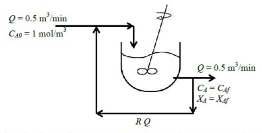
It is observed that when the recycle ratio R = 0.5, the exit conversion  $X_{Af} = 50\%$ . When the recycle ratio is increased to R = 2, the new exit conversion (in percent) will be:
