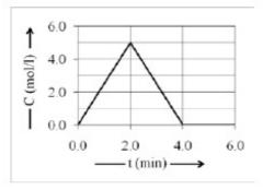
In the above figure, C is the exit tracer concentration. The corresponding *E* or  $E_{\theta}$  (normalized E) curve is correctly represented by which of the following choices ? Here,  $\theta$  is dimensionless time.
