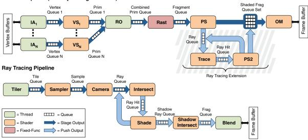
Direct3D Pipeline (with ray tracing extension)
