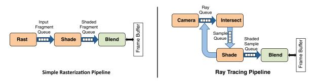
Fig. 1. Simplified GRAMPS graphs for a rasterization-based pipeline (left) and ray tracer (right). The ray tracing graph contains a loop. The early stages are automatically instanced for parallelism, while the Blend stages are both singletons to provide frame buffer synchronization.
