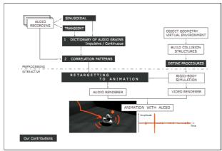
Fig. 3: Grain analysis and decomposition into sinusoidal and transient components[2]
