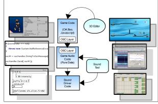
Fig. 5: Dataflow in Unity to Pure Data patch via OSC
