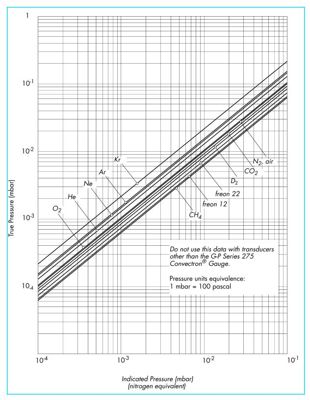
Figure 3-6 Convectron Gauge Indicated vs. True Pressure Curve; 10<sup>-4</sup> to 10<sup>-1</sup> mbar.
