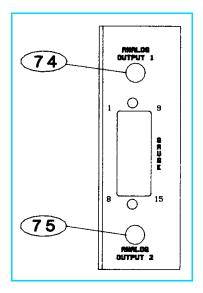
**Figure 4-2** Thermocouple Gauge Module Rear Panel.
