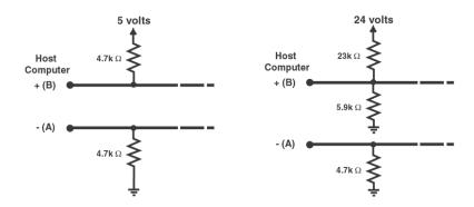
Figure 7-3 RS-485 Bias Resistor
