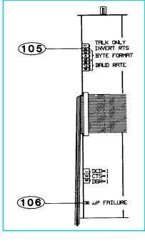
Figure 6-2 RS-232 Module, Top View.
