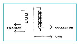
The filament is heated by direct current to such a temperature that electrons are emitted, and accelerated toward the grid by the potential difference between the grid and filament. All the electrons eventually collide with the grid, but many first traverse the region inside the grid one or more times.
