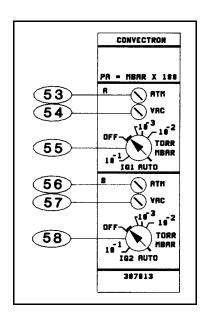
Figure 3-11 Convectron Module Front Panel.
