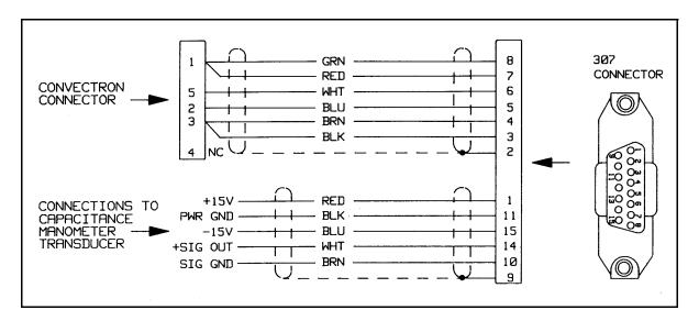
Figure 11-7 Capacitance Manometer Module Cable
