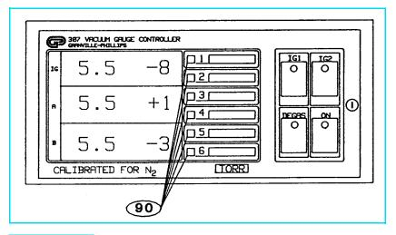
Figure 5-2 Process Control Relay Status Lights.
