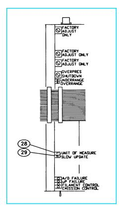
Figure 2-1 Ion Gauge Electrometer Module, Top View.
