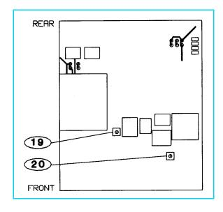
**Figure 1-13** Grid Voltage Adjustment, Power Supply PC Board.
