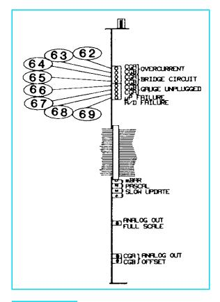
Figure 3-14 Convectron Module, Top view.
