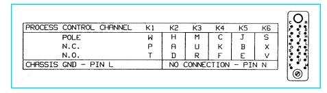
Figure 5-1 Pin Assignments/Connector.
