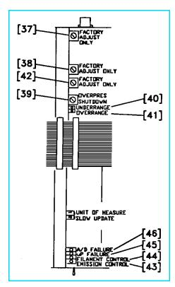
Figure 2-5 Ion Gauge Electrometer Module, Top View.
