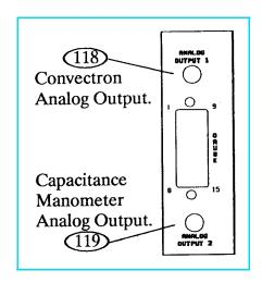
Figure 9-4 Capacitance Manometer Module, Rear Panel.
