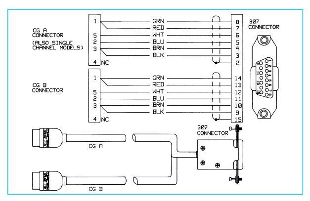
Figure 11-5 Convectron Gauge Cable
