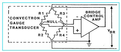
Figure 3-13 Simplified Schematic Convectron Gauge Module.
