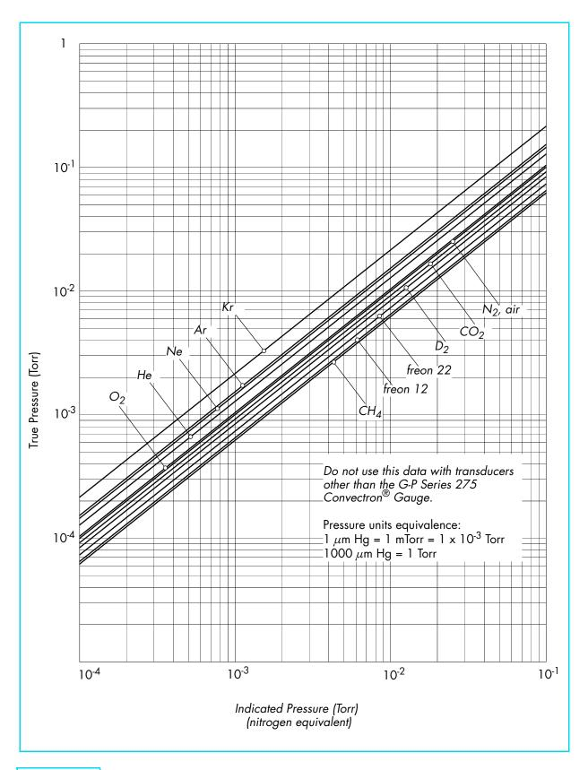
Figure 3-3 Convectron Gauge Indicated vs. True Pressure Curve; 10<sup>-4</sup> to 10<sup>-1</sup> Torr.
