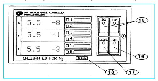
Figure 1-10 307 VGC Control Unit Front Panel.
