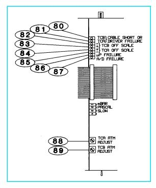
Figure 4-5 Thermocouple Gauge Module, Top View.
