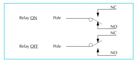
Figure 5-5 Process Control Relay Contacts Status.
