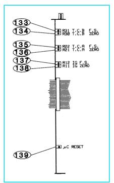
Figure 10-2 Linear Analog Output Module, Top View.
