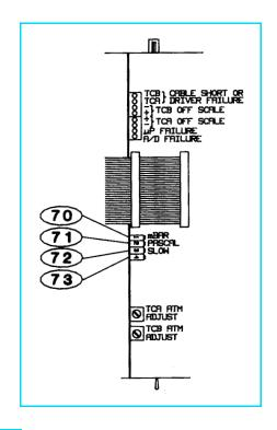
Figure 4-1 Thermocouple Module, Top View.
