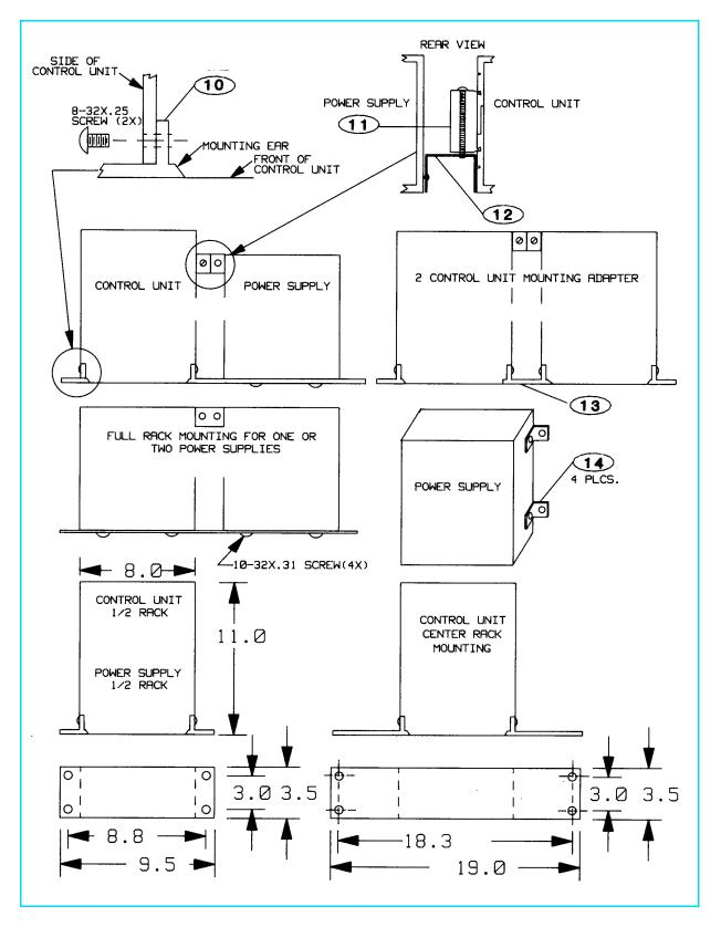
Figure 1-5 Mounting Methods.
