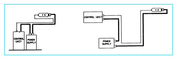
Figure 1-8 Collector Cable Routing.
