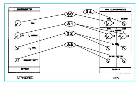
Figure 2-2 Electrometer Module Front Panel.
