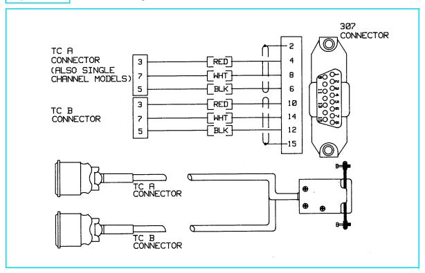
Figure 11-6 Thermocouple Gauge Cable
