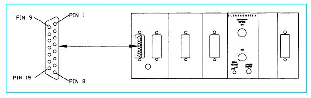
Figure 1-11 Remote Control Connector.
