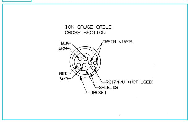
Figure 11-4 Ion Gauge Cable Cross Section
