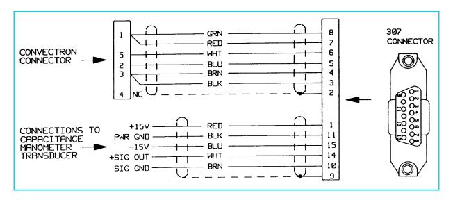
Figure 9-3 Capacitance Manometer Module, Cable.
