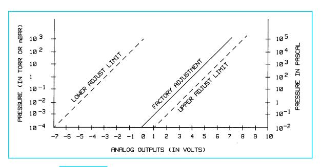
Figure 3-10 Convectron Gauge Pressure Analog Output.
