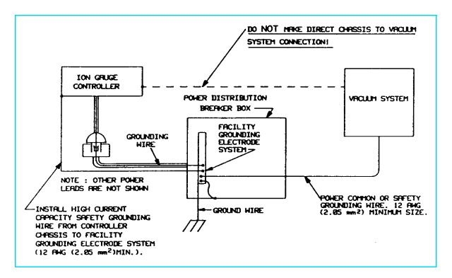
Figure 1-9 Correct System Grounding.
