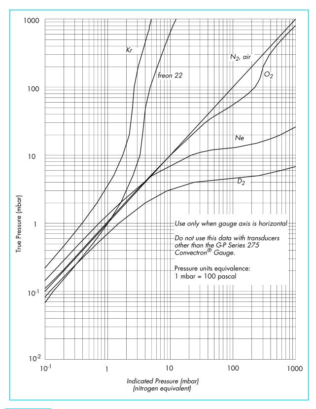
Figure 3-8 Convectron Gauge Indicated vs. True Pressure Curve; 10<sup>-1</sup> to 1000 mbar.
