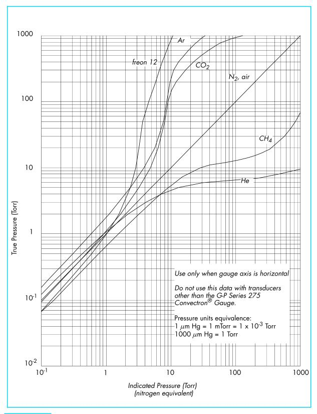
Figure 3-4 Convectron Gauge Indicated vs. True Pressure Curve; 10<sup>-1</sup> to 1000 Torr.
