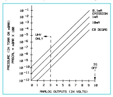
Figure 2-4 Ion Gauge Pressure Analog Output.
