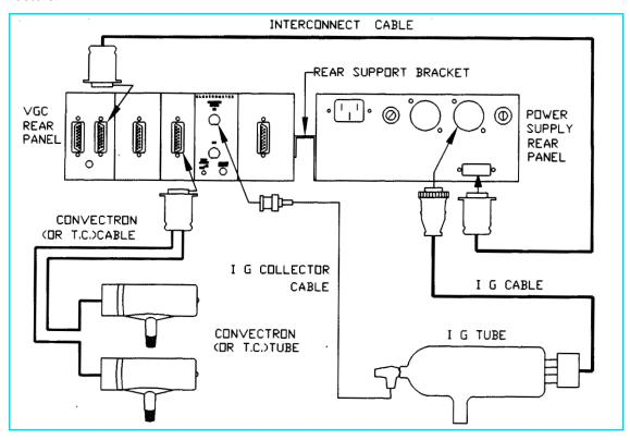
Figure 1-7 307 VGC Cable Connections.
