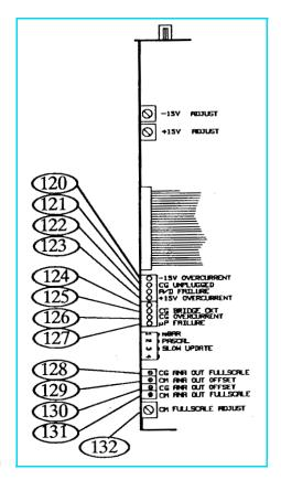
Figure 9-5 Capacitance Manometer Module
