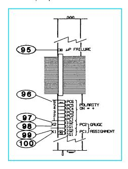
Figure 5-4 Process Control Module, Top View.
