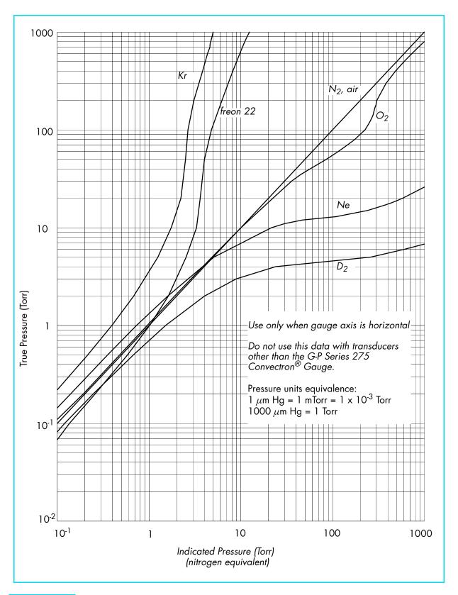
Figure 3-5 Convectron Gauge Indicated vs. True Pressure Curve; 10<sup>-1</sup> to 1000 Torr.
