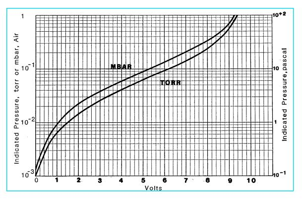
Figure 4-3 Thermocouple Gauge Pressure Analog Output.
