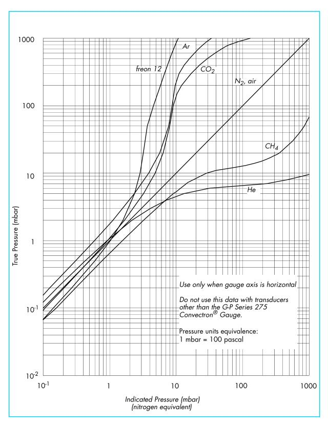
Figure 3-7 Convectron Gauge Indicated vs. True Pressure Curve; 10<sup>-1</sup> to 1000 mbar.
