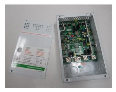
**Step 4:** Use the 5-foot red & black cable pair to connect your positive and negative battery terminals to the "Battery Positive" (use red cable from the positive battery terminal) and "Common Negative" (use black cable from the negative battery terminal) inputs of the C35 charge controller. It does not matter which Common Negative input you use.
