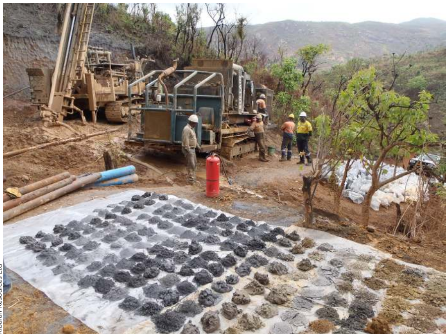
Figure 3: RC chip samples at Kibaran Resources Ltd's Epanko graphite project, Tanzania
