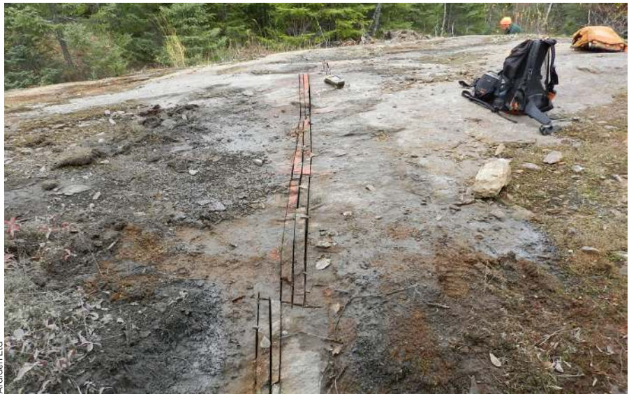
Figure 2: Channel sampling of a graphitic outcrop in Canada
