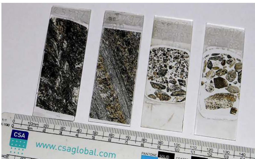
Figure 6: Polished thin sections. DD core on the left, RC chips on the right
