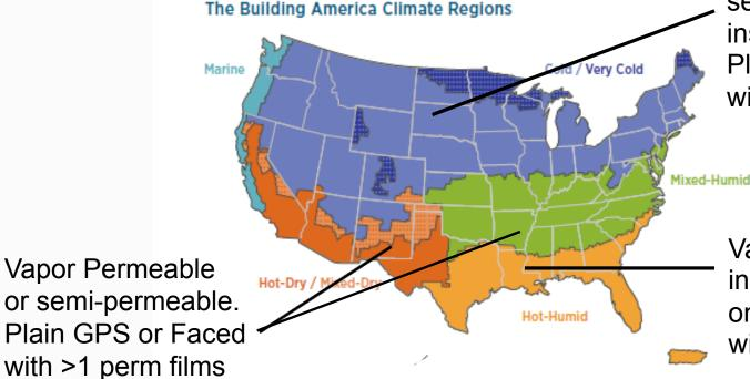
Vapor permeable or semi-permeable insulating sheathing. Plain GPS or Faced with >1 perm films.
