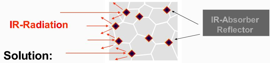
Incorporation of small quantities of highly effective Infrared-Absorbers/ Reflectors into the Polymer.
