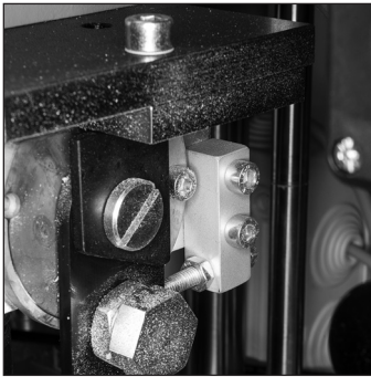
Hand lever adjusting screw. (front to back)
