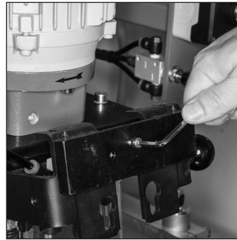
Side-to-side adjustment on ID arm plate.
