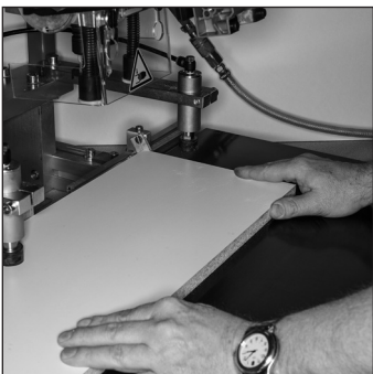
Press workpiece against the stop.
