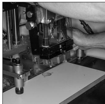
Press hand lever downwards.
