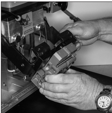
Fit ID onto bottom of ID arm
