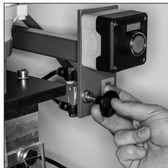
Clamp the hold-down devices.
