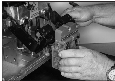
Angle ID to "hook" onto the ID arm
