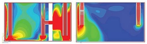
Figure 2. Comparison of Fluid Velocities in Single-Compartment and Two-Compartment Tank When Narrow Transfer Baffle is Used. Fluid velocity is indicated by color (blue is slow, red is fast). *Figure courtesy of the Water Environment Research Foundation*
