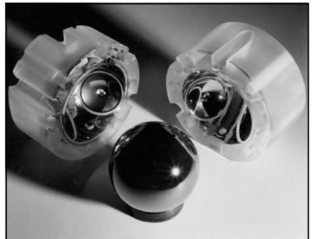
Gravity Probe B gyroscope (rotor) with quartz housing halves. Each milky-colored quartz rotor is coated with a sliver-thin layer of niobium, a superconducting metal. Inside each housing, six electrodes electrically suspend the gyroscope allowing it to spin freely at 4,000 rpm. Channels are cut in the quartz housing to allow helium gas to start the rotor spinning. A wire loop embedded in the housing acts as a SQUID to detect any change in direction of the gyroscope's axis.
