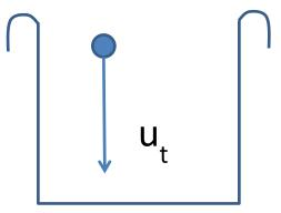
The heavier dispersed phase begins to drop with an acceleration but soon slows to a constant velocity, u<sub>t</sub>.
