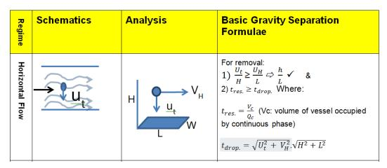
As it can be seen, there are two criteria which should be met to make sure separation happens:
