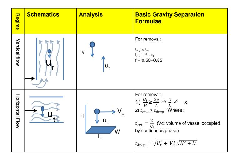
The above equations are for gravity separation. However, a gravity separator shouldn't necessarily be designed solely on the basis of the equations of gravity separation. Other important parameters are involved which affect the design. Sometimes these parameters function as a complementary equation in the design, or are used in the place of portions of the gravity separation equations.
