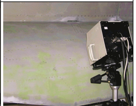
Figure 57. FTIR operating on a camera tripod to analyze the F-16.
