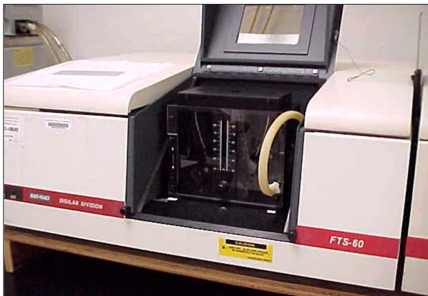
Figure 3. FTIR with variable-angle sampling device.
