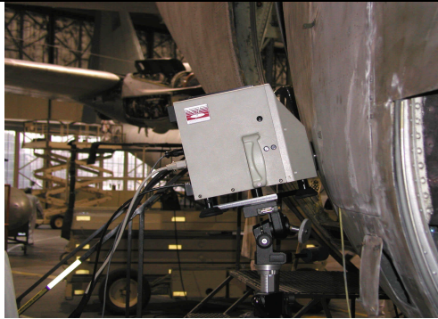
Figure 50. FTIR analyzing C-130 bare aluminum belly.
