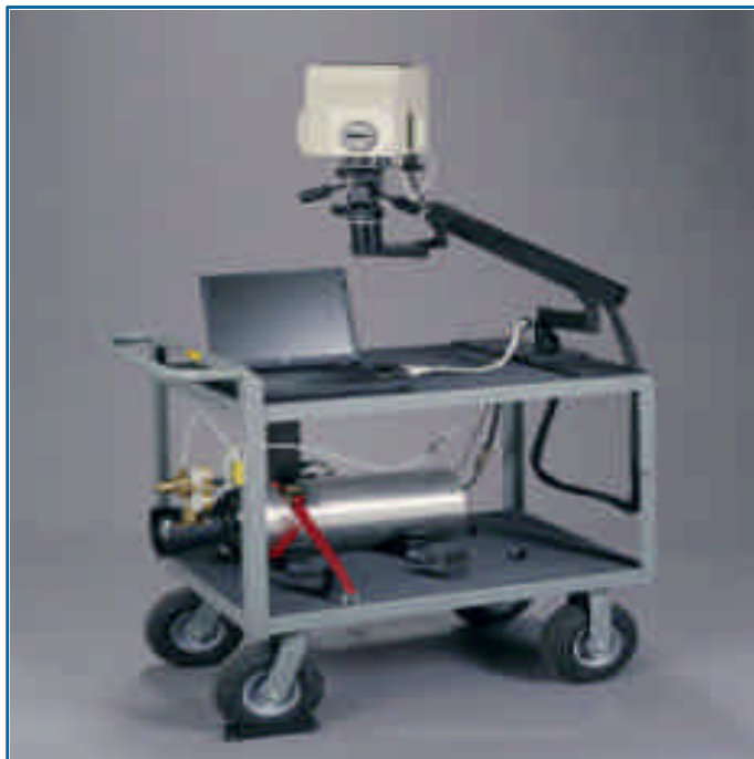
Figure 19. Portable grazing-angle FTIR prototype with computer and cart assembly.
