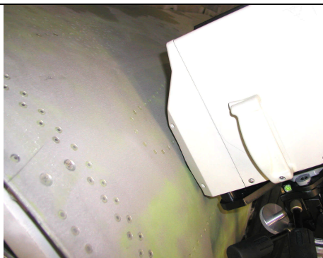
Figure 55. Close-up of the FTIR analyzing an F-16 landing gear door.
