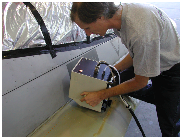
Figure 41. Close-up of the FTIR device sampling a wing awaiting final coating application after cleaning and conversion coating.
