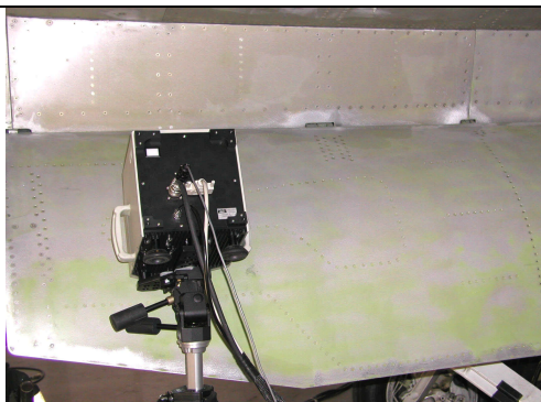
Figure 56. FTIR analyzing an area containing yellow epoxy primer.
