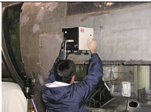
Figure 53. FTIR operator at the C-130 demonstrating hand-held FTIR operation.
