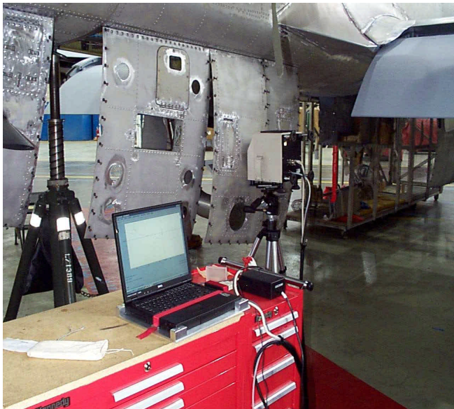
Figure 45 . FTIR unit sampling a landing gear door. Laptop computer controller is in the foreground.
