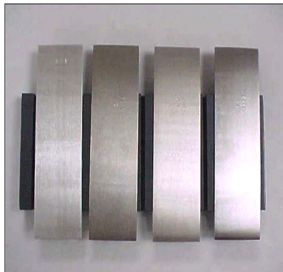
Figure 5. Aluminum, titanium, stainless steel, and steel alloy (from left to right, all at 600-grit).
