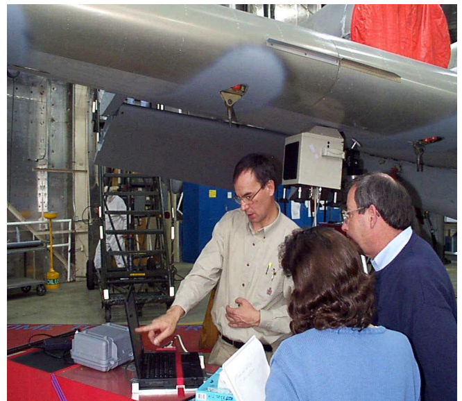
Figure 48. Operators observe collection of data by the FTIR and instantaneous conversion of data to a spectrum on the computer screen.
