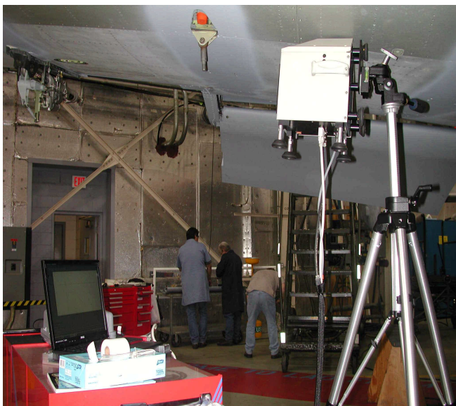
Figure 47. Reorientation of FTIR device on the tripod to analyze the underside of a wing.
