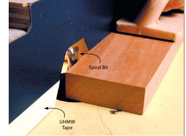
wears forever and provides a slick surface for the wood to glide on. Using a straightedge, set the fence so the cutter is exactly flush with the taped side.
