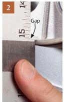
Measure the gap with a ruler calibrated to at least 1/32 in. or with a dial caliper.
