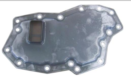
After the automatic transmission hydraulic system components have been in use for a long time, the fluid may deteriorate or be polluted by dust particles in the air due to wear particles of parts, friction lining peeling off or excessive wear of seal, which may cause stuck slide valve and blocked orifice. Therefore, strict measures should be taken to filter the fluid.
