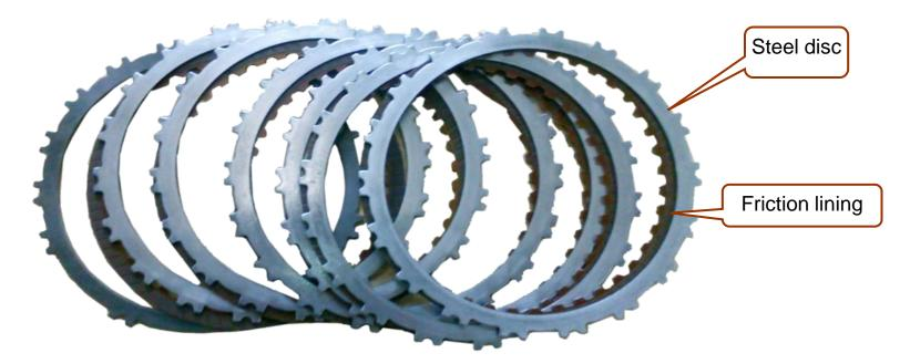
The disc brake (equivalent to the clutch drum) is fixed on the automatic transmission housing; when the brake operates, certain element in the planetary gear set connected with the brake hub will be fixed and cannot rotate.
