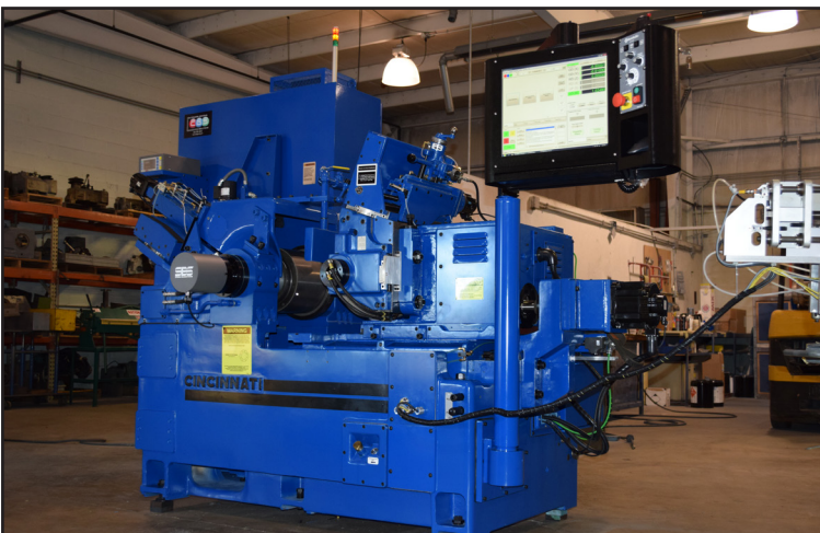
Cincinnati Centerless Grinder Controller
