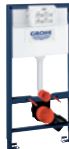
38 525 001 Rapid SL for WC with flushing cistern 6 – 9 l dual flush/start & stop/single flush, 1.00 m installation height connection from left/right/rear actuation from front/above
