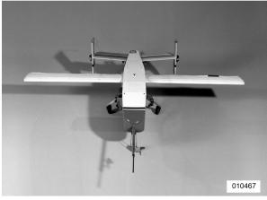
Figure 10. Photo comparison of I-2000 with wings stowed (top) and inflated (bottom).
