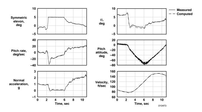
Figure 16. Comparison of flight-measured and computed time history results for a POPU maneuver in the preinflated-wing configuration.
