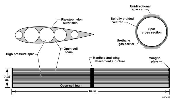
Figure 1. Inflatable wing structure.
