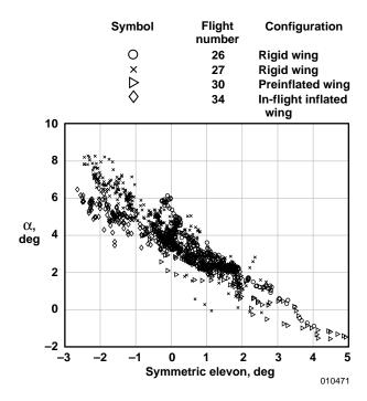
Figure 14. Trim curve for three configurations.
