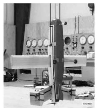
Figure 12. Test configuration for inertia swing on I-2000 (suspension lines exaggerated for clarity).
