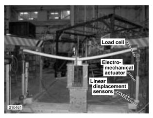
Figure 3. Static structural testing of the inflatable wing.
