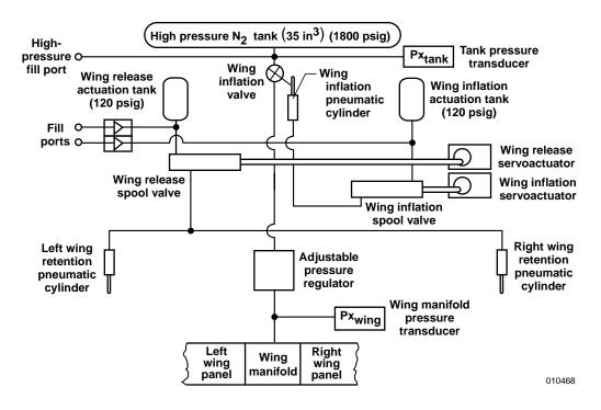
Figure 11. Schematic of the integrated in-flight-inflation system.
