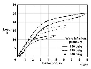
Figure 4. Left wingtip load as a function of wingtip deflection.
