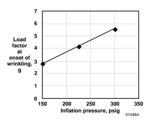
Figure 6. Allowable load factor as a function of wing inflation pressure.
