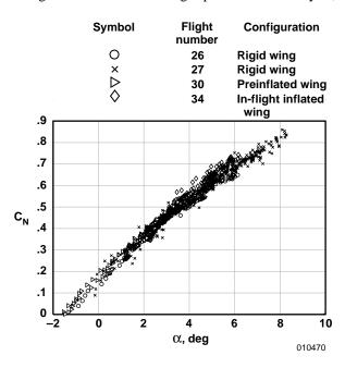
Figure 13. Normal force coefficient as a function of  $\alpha$  for three configurations.
