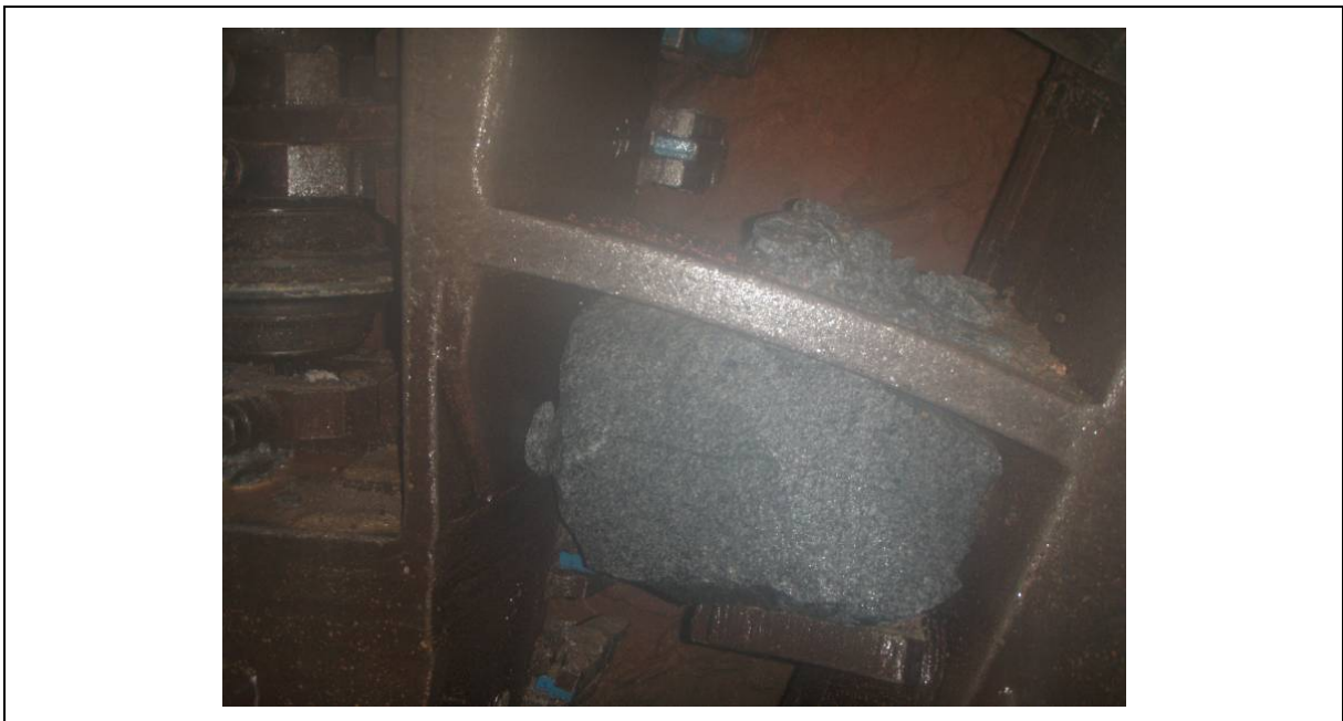
Figure 8.2 Example of Rock Fragment Trapped in the Cutterhead
