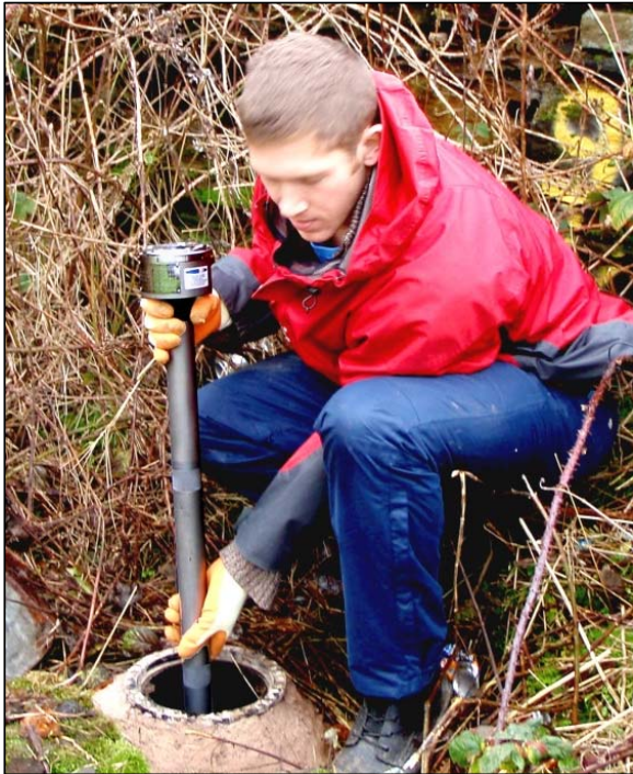
1 st Generation In-borehole device GasClam ®
