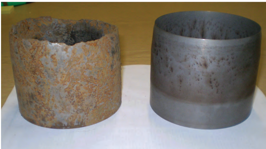
Figure 1: deformation of thin-walled cutting shoe in stony glacial till
