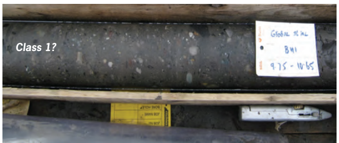
Figure 7: very stiff glacial till obtained by triple-tube rotary core Geobore S drilling
