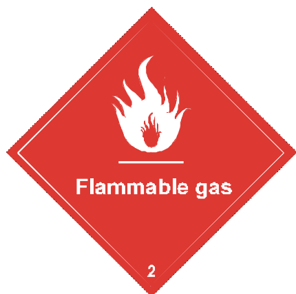
figure 8 hazard label - flammable gas
