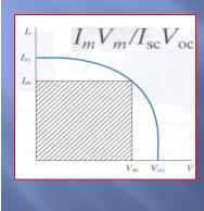
Q3. This figure shows the fourth quadrant portion of a solar cell characteristic, with Ir plotted upward for convenience of illustration. A Si solar cell has a Isc = 100mA, Voc = 0.7V under solar illumination. The ratio ImVm/IscVoc is 0.7. What is the maximum power delivered to a load by this cell? (Hint: Pmax = fill factor\*Isc\*Voc)
