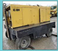
Sullair Model 750-DP Trailer Mount Diesel Power Portable Air Compressor
