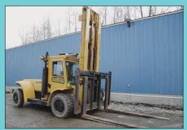
30,000 Lb Hyster H300B Dual Pneumatic Tire Diesel Power Lift Truck
