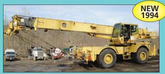
Grove Model RTC-635C 4X4 Hydraulic Rough Terrain Crane
