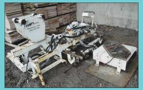
Minnich Model H-3 Three-Spindle Gang Drill Attachment
