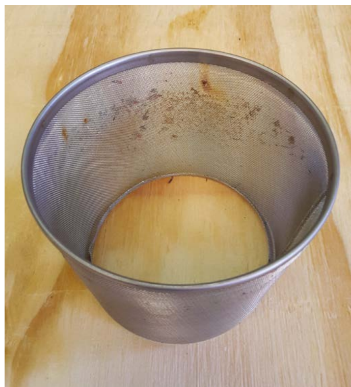
Figure 4. Basket filter removed from the unit head of the proportional dilutor ready for cleaning
